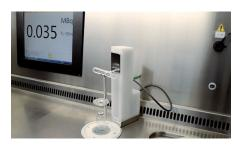
**Dose calibrator\*** - The ionisation chamber compartment is at the centre of the machine work surface. The sample holder lifter automates the lifting action of the vials/syringes from the ionisation chamber to the work surface and vice-versa.
