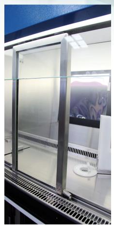
**Sliding Lead glass window\*** to protect the operator from radiation.
