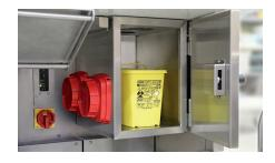
**Solid waste compartment\*** - The waste is stored in the compartment through an opening on the work surface. The waste is then removed through the shielded front door. This process follows the GMP guidelines, according to which, the waste must not be removed directly from the sterile work area.
