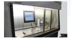
**Work chamber** - Spacious work chamber made of AISI 304 stainless steel for maximum ergonomics, equipped with a motorised safety 8 mm thick glass window. A 17" monitor integrated in the rear side of the work area, used to control the dose calibrator\*.
